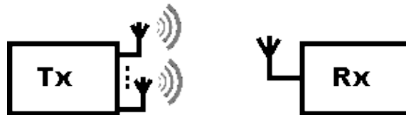
Fig 4.3: Multiple Input Single Output ( MISO )
