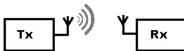
Fig 4.1: Single Input Single Output ( SISO )
