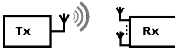
Fig 4.2: Single Input Multiple Output ( SIMO )
