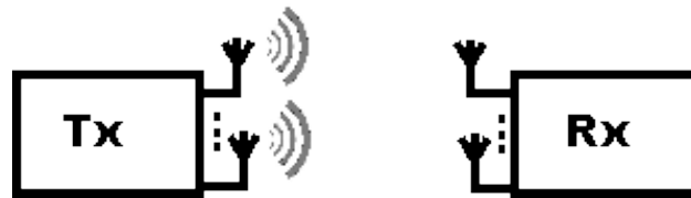
Fig 4.4: Multiple Input Multiple Output ( MIMO )
